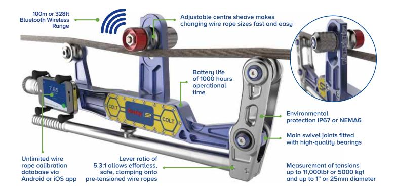
The Straightpoint COLT is a lightweight wire rope tension meter, for fast and accurate measurement of tensions up to 11,000lb or 5000 kg and up to 1" or 25mm diameter.
