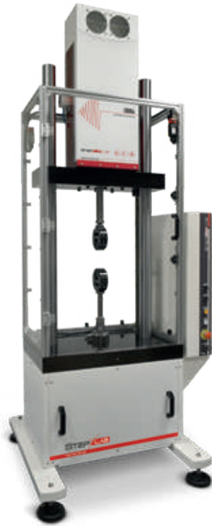
Application of the linear motor actuator UD04
