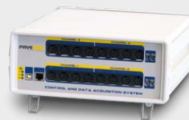
CDAS Control and Data Acquisition System
