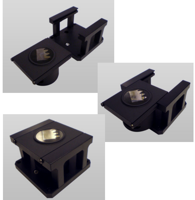
Fig. 2: Specimen mount: separate, sliding in, closed up
