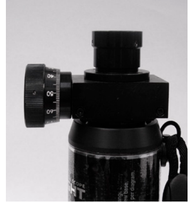
HiLight Microscope with optional integral micrometer
