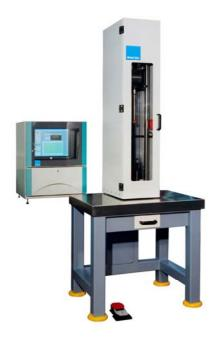
A dedicated system for the multi-axial impact testing of plastic and composite plaques to defined quality standards such as: ISO6603, ISO7765 and ASTM D5628.
