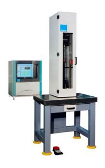
A dedicated system for the multi-axial impact testing of flexible sheet film to defined quality standards: ASTM D1709, DIN53373, BSI 2782 method 352D and ISO EN 7765.
