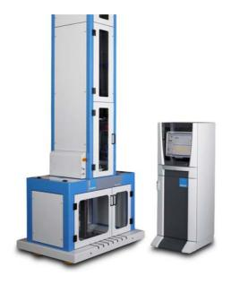
A highly versatile range of drop weight impact testers for performing a wide range of medium energy tests on materials, specimens and end products of various geometry.
