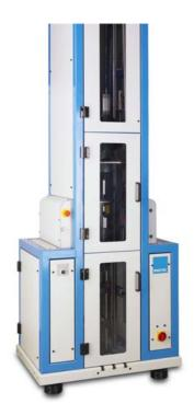
A highly versatile range of drop weight impact testers for performing a wide range of medium energy tests on materials, specimens and end products of various geometry.
