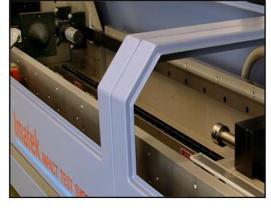
Applications include plaque and film testing, automated testing for quality assurance purposes, characterisation of energy-absorbing materials, resilience testing of rubbers, low-energy testing of advanced composites, high-rate tensile testing, Charpy and IZOD testing and fatigue testing.
