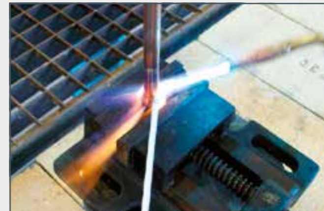
Heating the workpieces up to the soldering heat and melting of flux material and solder. By capillary effect solder automatically fills the soldering gap.
