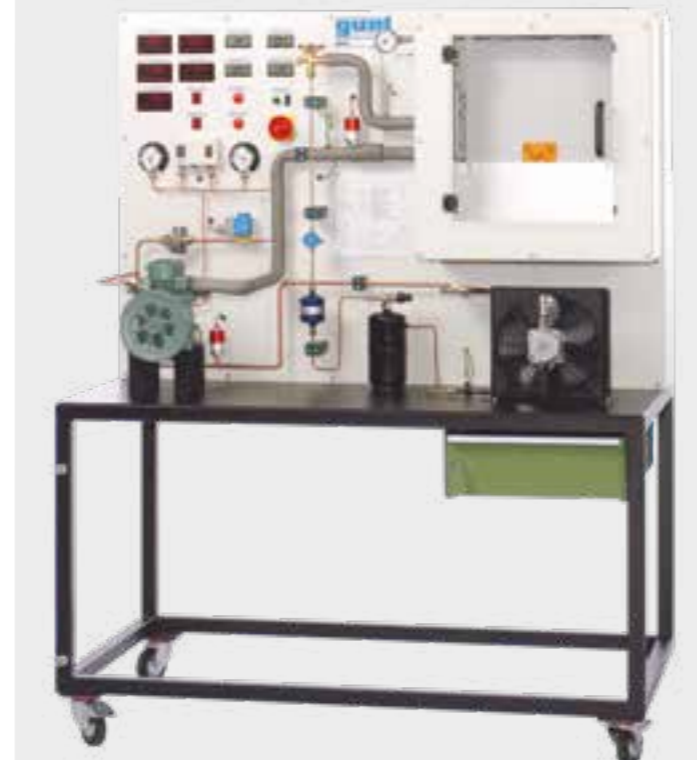
ET 165 Refrigeration system with open compressor
