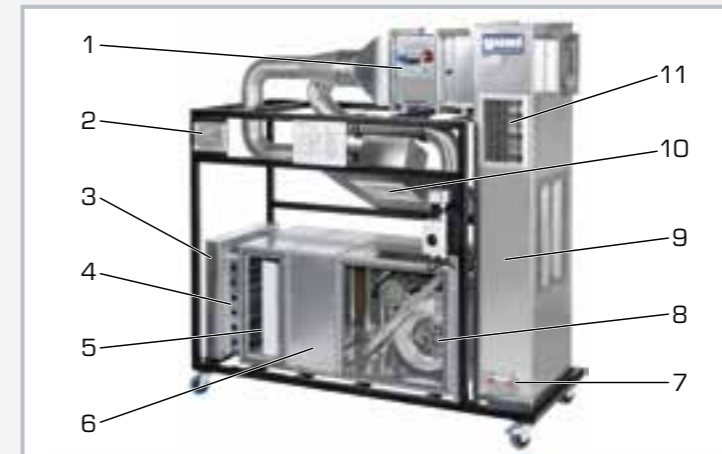
1 fire protection flap, 2 inclined tube manometer, 3 weather louvre, 4 multi-leaf damper, 5 filter, 6 heat exchanger, 7 inspection cover, 8 fan with drive motor, 9 air duct, 10 ceiling vent, 11 wall vent
