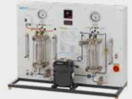
ET 350 for demonstration of the processes in a refrigeration circuit
