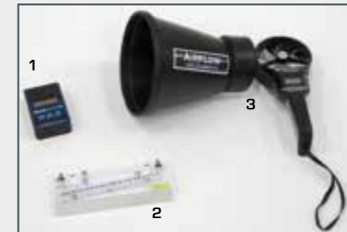
1 digital manometer, 2 inclined tube manometer, 3 anemometer
