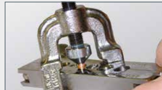
Flaring of the pipe with the flaring tool
