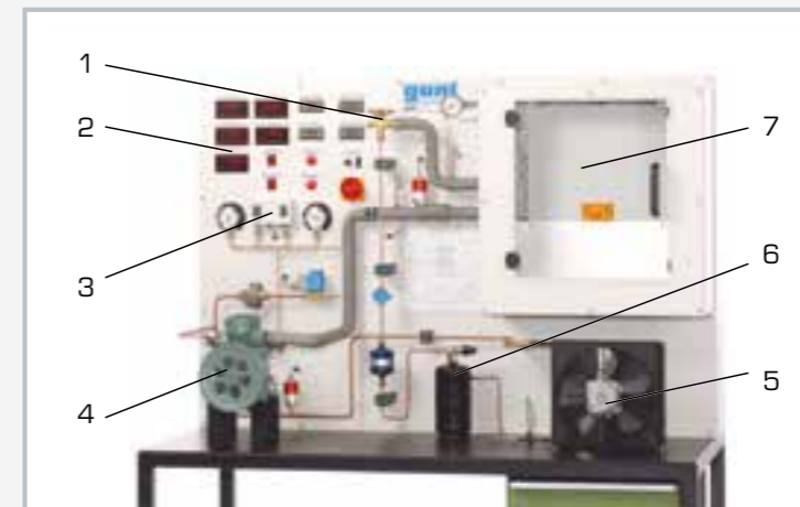
1 expansion valve, 2 displays and controls, 3 pressure switch, 4 compressor, 5 condenser, 6 receiver, 7 refrigeration chamber
