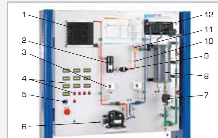
1 condenser with fan, 2 receiver, 3 high pressure switch, 4 displays and controls, 5 heater controller, 6 compressor, 7 pump, 8 warm water tank with heater, 9 filter/drier, 10 sight glass, 11 expansion valve, 12 evaporator
