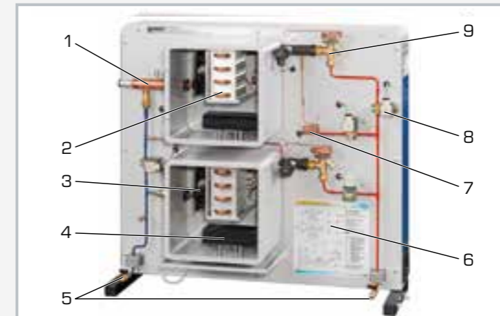
1 evaporation pressure controller, 2 evaporator, 3 fan, 4 heater, 5 connections to ET 915, 6 process schematic, 7 capillary tube, 8 solenoid valve, 9 expansion valve
