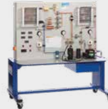
ET 411C represents a typical compression refrigeration circuit
