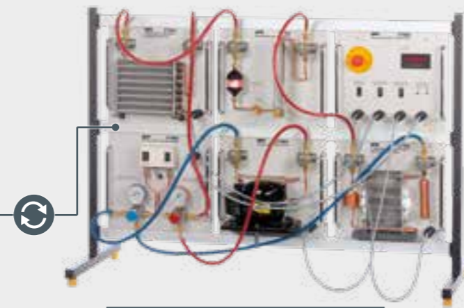
Components arranged in a frame and connected with refrigerant hoses
