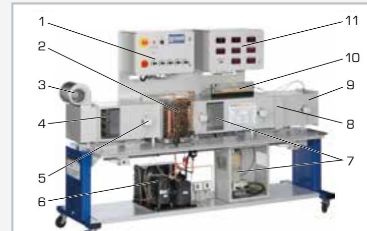
1 controls, 2 air cooler (direct evaporator), 3 fan, 4 air preheater, 5 temperature sensor, 6 condensing unit, 7 air humidifier, 8 air reheater, 9 air duct, 10 inclined tube manometer, 11 displays
