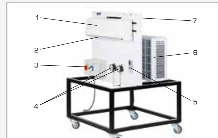
1 air inlet inner unit, 2 air outlet inner unit, 3 switch cabinet, 4 manometer, 5 remote control, 6 outer unit, 7 dividing wall
