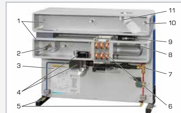
1 air duct, 2 air reheater, 3 process schematic, 4 air humidifier, 5 connections for ET 915, 6 evaporator, 7 expansion valve, 8 air preheater, 9 fan, 10 sensors for humidity and temperature, 11 ventilation flap
