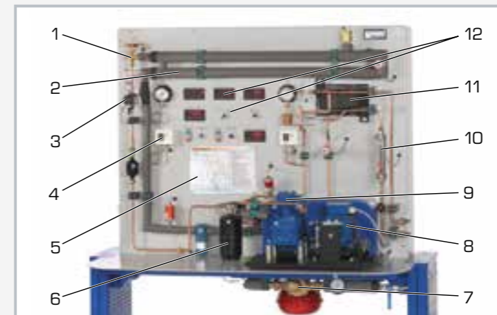
1 expansion valve, 2 evaporator, 3 refrigerant flow meter, 4 pressure switch, 5 process schematic, 6 receiver, 7 hot water circuit of the evaporator, 8 drive motor, 9 compressor, 10 cooling water flow meter, 11 condenser, 12 displays and controls
