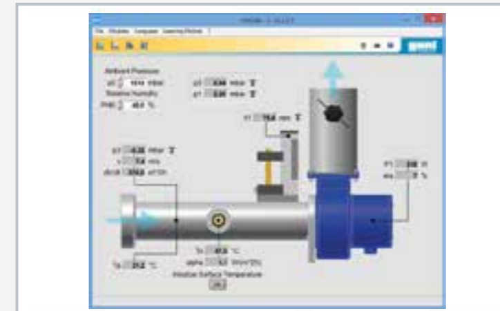
Screenshot of the software together with the electronic total pressure sensor accessory HM 240.03 and pressure distribution on a cylinder HM 240.04
