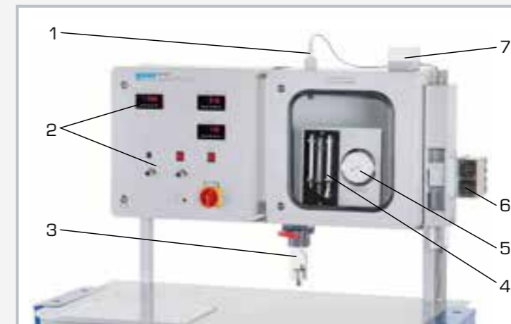
1 capacitive humidity sensor, 2 displays and controls, 3 humidifier, 4 psychrometer, 5 hair hygrometer, 6 dehumidifier, 7 hygrometer with synthetic fibre and combined temperature sensor
