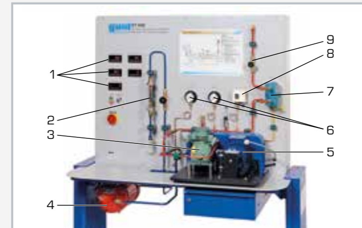
1 displays and controls, 2 flow meter, 3 refrigerant compressor, 4 stabilisation tank, 5 drive motor with torque measurement, 6 manometer, 7 oil separator, 8 pressure switch, 9 valve
