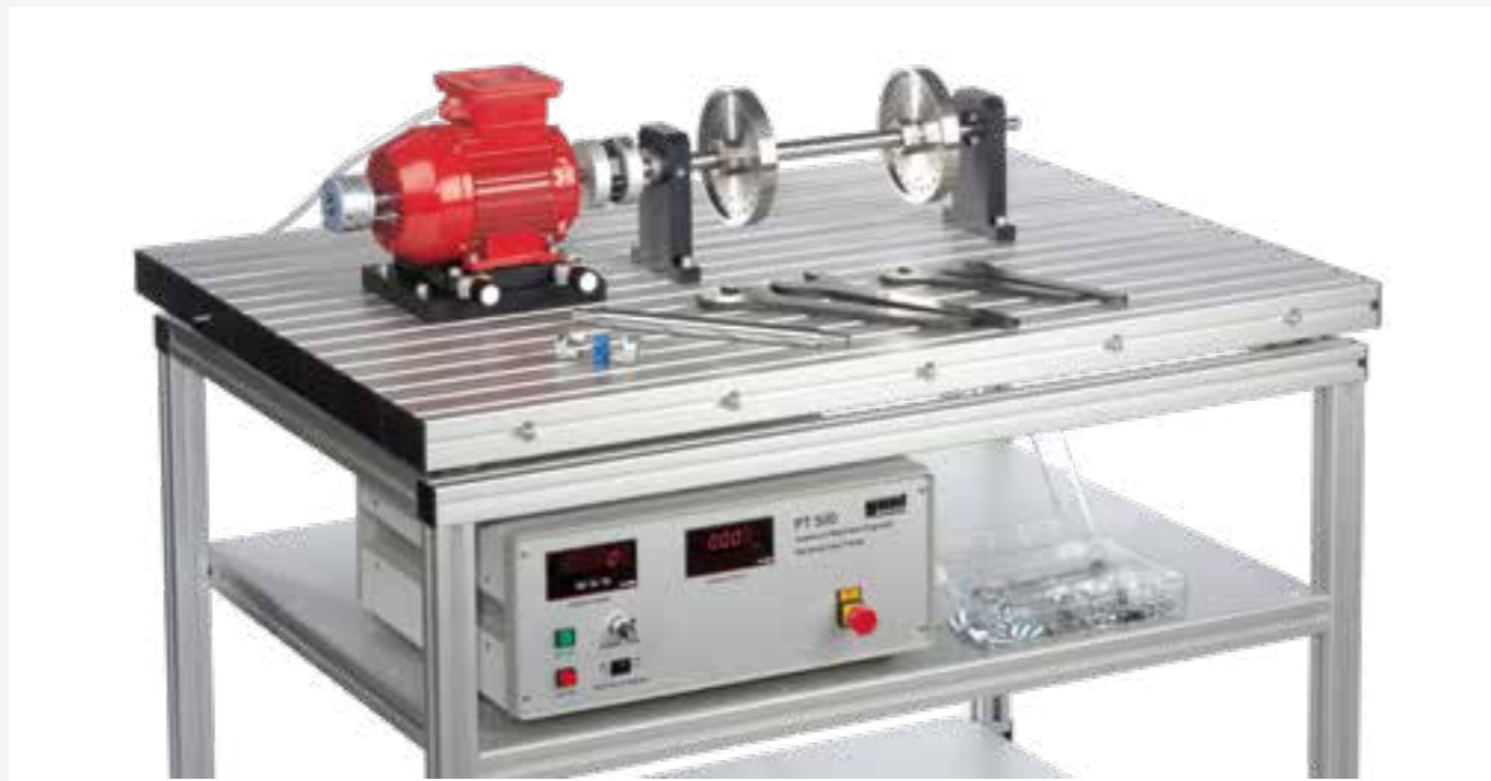
The illustration shows the base system PT 500 ready for conducting experiments, together with the trolley PT 500.01.
