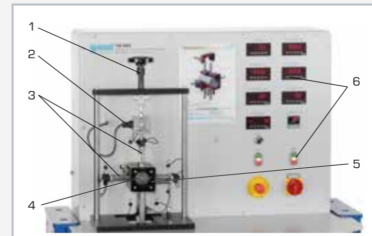
1 handwheel for load, 2 force sensor for frictional moment, 3 inductive displacement sensors, 4 shaft, 5 bearing housing, 6 displays and controls
