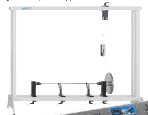
SE 110.19 Investigation of simple stability problems
