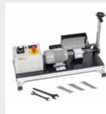
The compact WP 140 experimental unit is used to conduct fatigue strength tests
