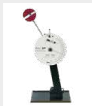
The WP 410 experimental unit generates a 300Nm work capacity
