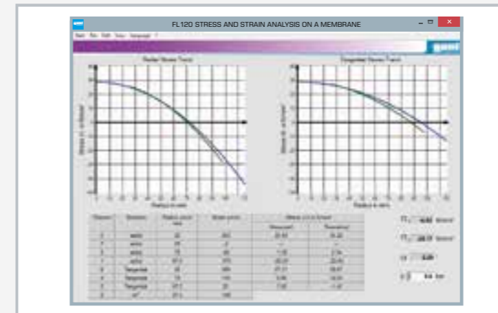
Application software for stress and strain analysis based on the example of the FL 120 (stress and strain analysis on a membrane)
