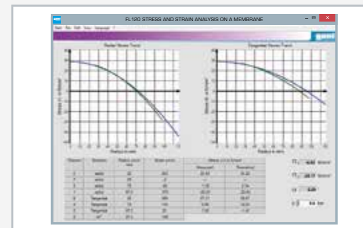
Application software in FL 152 for stress analysis: representation of the stress curve
