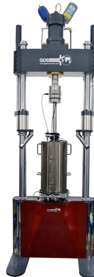
250kN Hydraulic Loading Frames (HLF)
