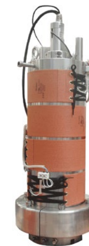
20MPa triaxial cell with heating pads 100mm max sample diameter
