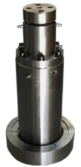
64MPa triaxial cell with balanced ram 100mm max sample diameter
