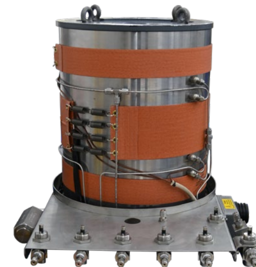
Instrumented Hoek Cell, shown with heat pads (GDSIHC)
