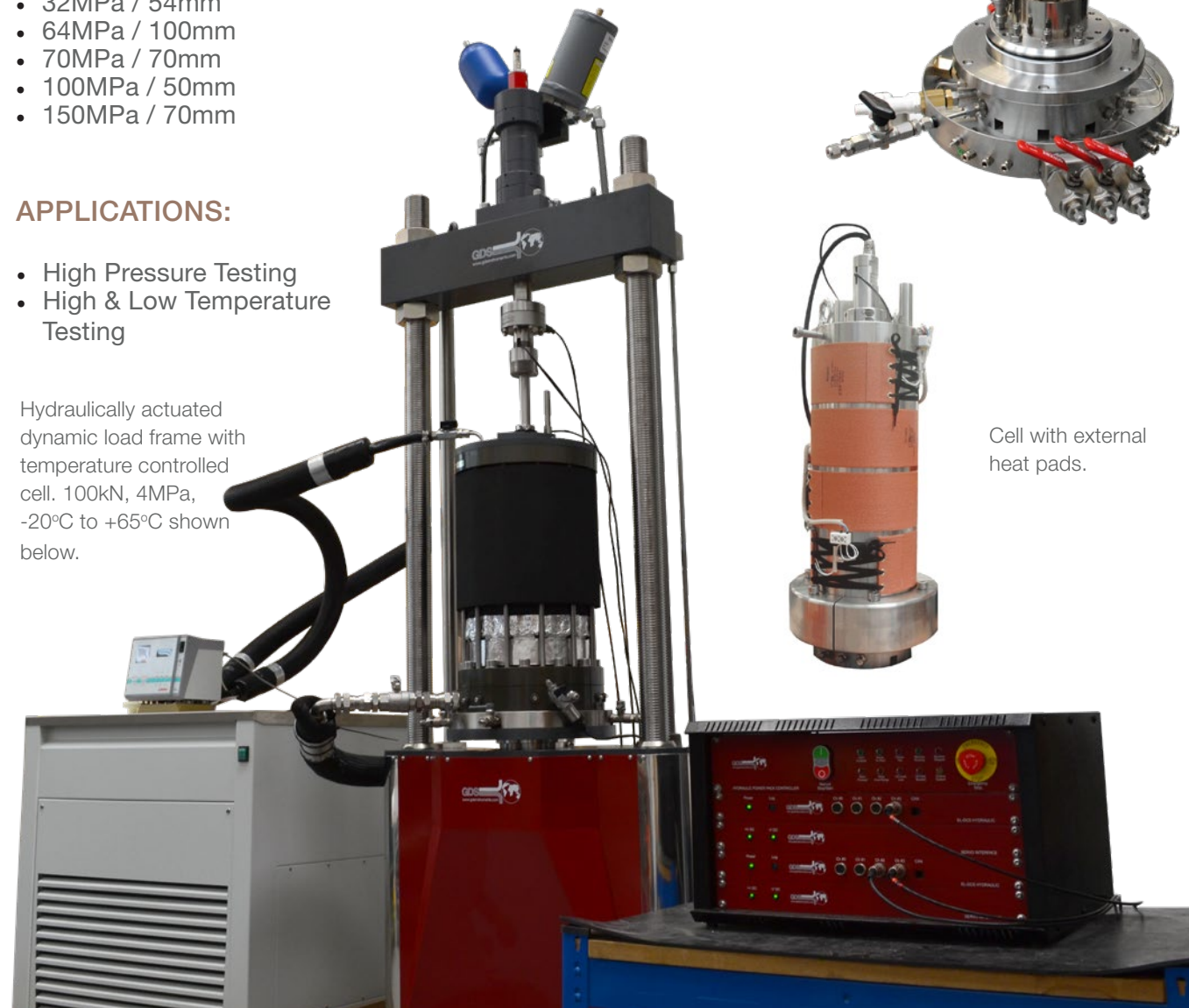
Cell base with heating and cooling coil.
