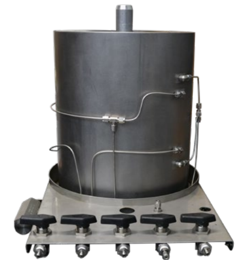
Instrumented Hoek Cell (GDSIHC)
