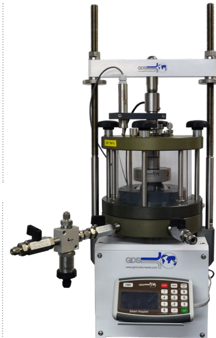
Constant Rate of Strain (CRS) Testing, with elevated back-pressure in 10kN loadframe.
