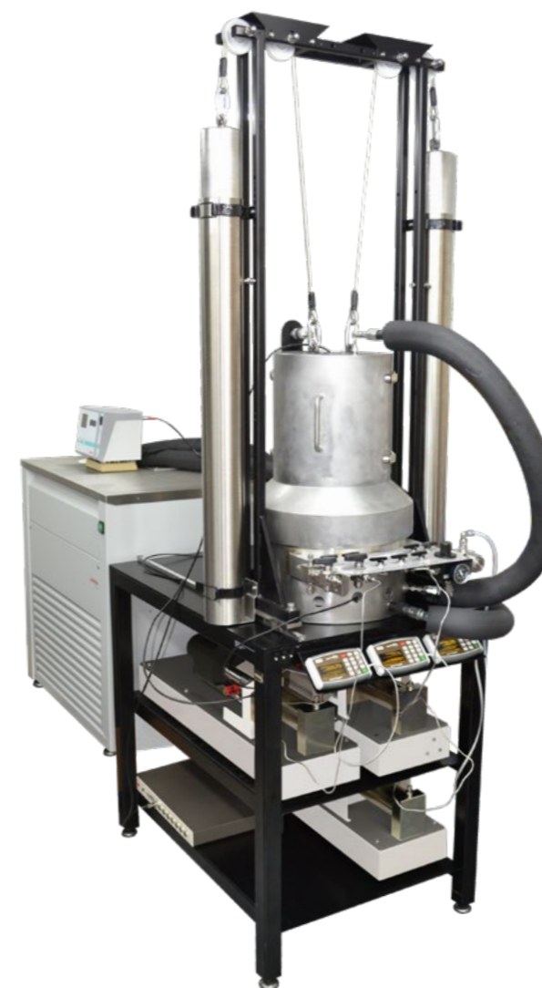
The Environmental Triaxial Testing System (ETTS) is a temperature controlled testing system for stress path testing.
