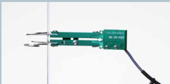
Model 3442 with 6.0 mm gauge length and +5.0 mm/-1.0 mm (+83%/-17% strain) measuring range
