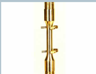
Laser extensometer high temperature clip-on reflectors
