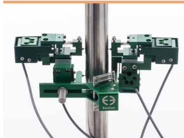
Model 3550 axial/torsional extensometer with a 25 mm gauge length, \pm 10\% axial measuring range, and \pm 2^\circ torsional shear strain angle measuring range (this corresponds to a 4^\circ angle of twist on a 12.5 mm diameter specimen)
