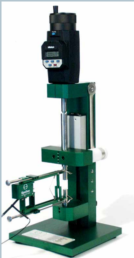
Model 3590 calibrator with Model 3542 axial extensometer
