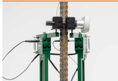
Model 3567 specimen attachment collar with extensometer installed
