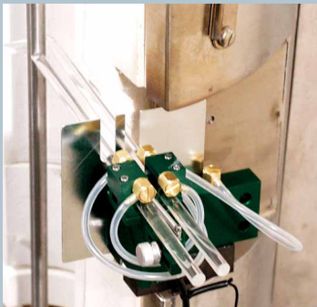
Model 3580 mounted to split furnace
