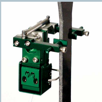
Model 3475-050T-ST with \pm 0.050 inch measuring range
